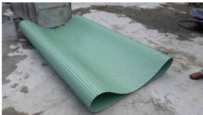
FIGURE 2: AKS HDPe Lining Prior to Casting into
